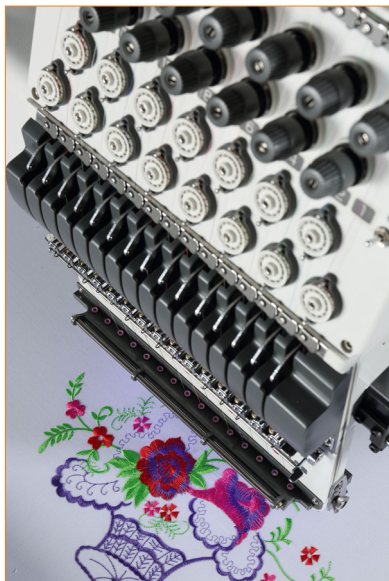
Tension arm guards for added safety
