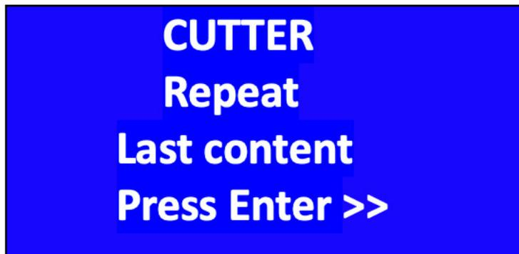
The cutter will remember the last job sent from the computer to the cutter. To re-cut the previous design, press
